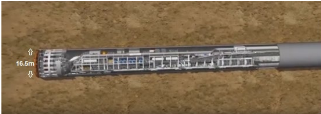
Plate 3.1 Cutaway view of a large diameter TBM (Herrenknecht)
